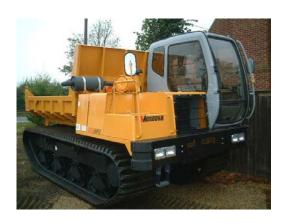
The Morooka Tracked Carrier features a very low ground pressure due to the rocking beam bogey track system. Fitted with a two speed hydrostatic transmission this provides excellent traction and power to the drive motors. The operator can be comfortable working in all climates thanks to the fully air conditioned cab with heater and tinted glass.
